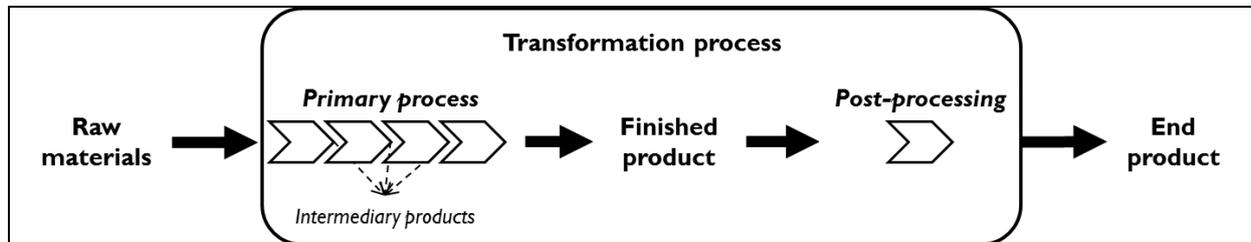
Figure 1: A simplified model of the material transformation process in process industries (adapted from Storm et al. (2013)).
