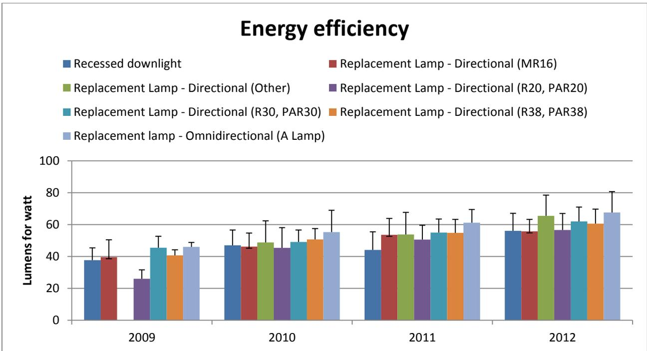
Figure 6 Energy efficiency dynamics in the lightingfacts database. Sample n=2,785 lamps (own elaboration)
